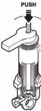
Tighten the cartridge with the shaft pressed and wipe the overflowed oil.
