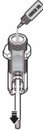
Pull down the piston to the bottom of cylinder and fill it two-thirds with oil.
