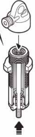
Push up the shock shaft slowly to the top and close the cap.
